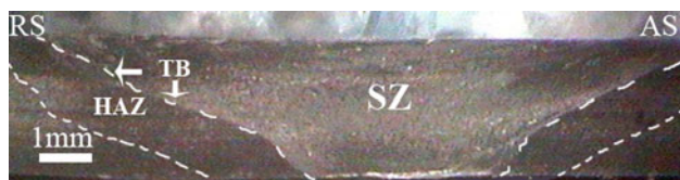
Fig. 10 Macroscopic view of the joint cross section in condition 4III
