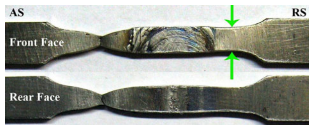
Fig. 14 The tensile specimen of condition 4III after tension test, fracture occurred in 17 mm away from the center of joint, necking (pointed by arrows) was happened in RS of the specimen as well
